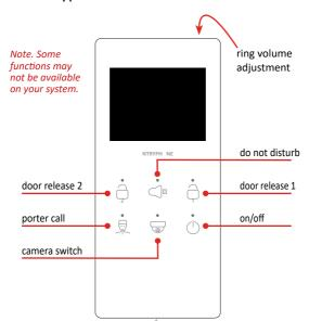
The Entryphone 516V is a wall-mounted, full duplex, loudspeaking, colour video telephone. The video screen turns on automatically when the telephone is called and the lamp above the on/off touch switch will flash. If you want to speak to the caller, press the on/off touch switch and this will enable the speech connection.
