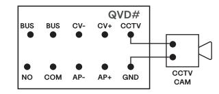
By default, Q series systems only display the caller at the door panel that initiated the call. However, you can add an additional camera at the door for a second view of the caller. Any video camera with a CVBS analogue output can be connected to the QVD's "CCTV" input. Note that additional cameras cannot be powered by the QVD and will require a separate power supply.
