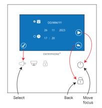
To adjust the time/date parameters first press the  $\bigcirc$  button to move the focus to either the date or time (the tick  $\bigcirc$  will move to indicate it is selected) and then press the  $\bigcirc \mathfrak{a}$  button to select.
