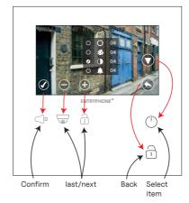
Use the  $\bigcirc$  button to move the focus (the tick  $\bigcirc$  will move to indicate what is selected) and then increase or decrease the setting, using the  $\bigcirc$  and  $\bigcirc$  buttons. As you change the brightness, colour or contrast the background on the screen will change accordingly. When changing the volume of the ringer the sound will play.
