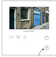
Press and hold the lock button until the brightness, colour, contrast and volume icons appear
