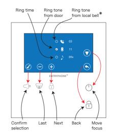
To change either the ring tone, or ring time, press the  $\bigcirc$  button to move the focus to that option (the tick  $\bigcirc$  will move to indicate it is selected). Use the  $\bigcirc$  and  $\bigcirc$  buttons to move to the next or last choice. With the ring tone you will hear the selected tone. Once satisfied with your selection press the  $\bigcirc$  button to confirm.
