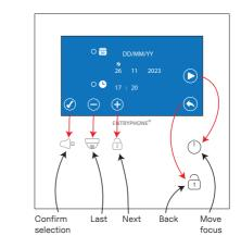
To adjust each number press the  $\bigcirc$  button to move the focus (the tick  $\checkmark$  will move to indicate what is selected) and then use the  $\bigcirc$  and  $\bigcirc$  buttons to change the number incrementally followed by the  $\bigcirc$  button to confirm.
