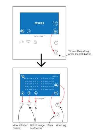
In the call history the most recent captured image is the first in the list and marked with a  $\bigcirc$ . To move the selection use the  $\bigcirc$  and  $\bigcirc$  buttons and then the  $\bigcirc$   $\bowtie$ to view your chosen image.
