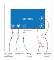
Within the settings menu, you can adjust various parameters such as the unit's time and date, configure picture and video memory settings, change the ring tone, and reset the unit to its factory defaults. Each process is described in detail in the following pages.
